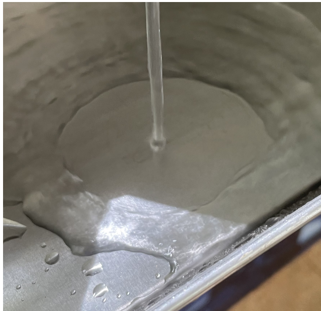
Fig. 1.1 Image of circular hydraulic jump in a water dispenser. Water jet hits the solid surface and a sudden increase in film thickness is observed at a fixed radial distance.
