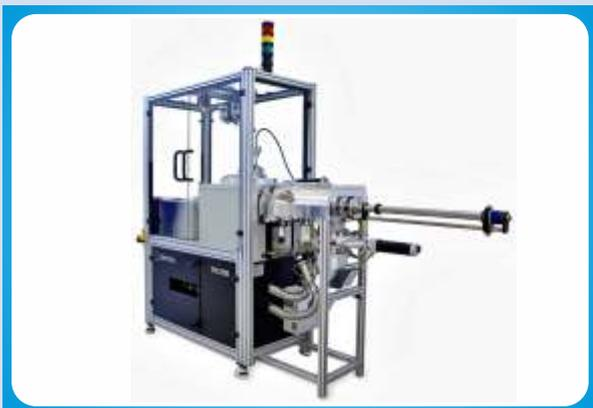
**Atomic Layer Deposition System (ALD), TFS 200** installed at Sheikh Saqr Laboratory at International Centre for Materials Science.
