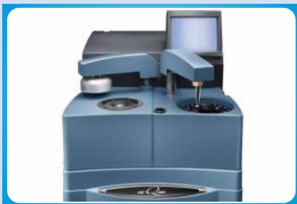
Q 2000 Modulated Differential Scanning Calorimeter (MDSC) System installed at Chemistry and Physics of Materials Unit.
