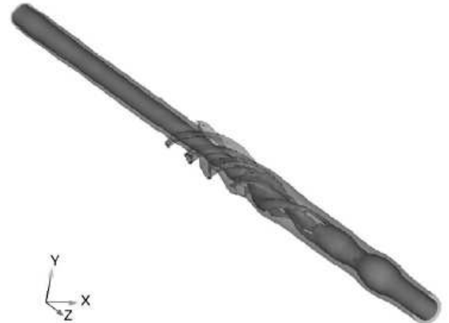
(b) Numerical evidence of ‘bursting’ of a trailing vortex (Moet et al. [2005])
