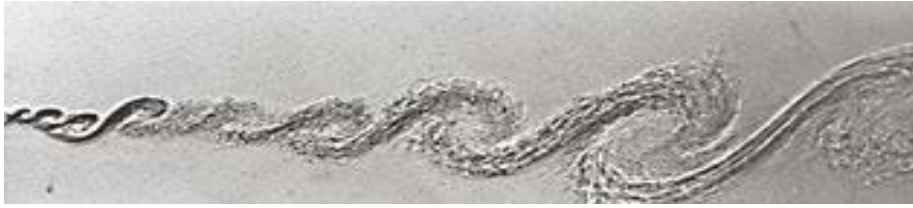
Figure 1.2. Large scale coherent structures in a turbulent mixing layer (Konrad, 1977)
