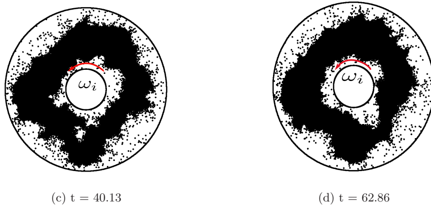
Figure 4.18: Snapshots showing different stages of cluster co-existence of gas + solid at different times marked in Fig. 4.17(a) (red points). Parameters are same as in Fig. 4.16 for \omega_i = 0.1 , d_w = 75 and e_n = 0.6 .
