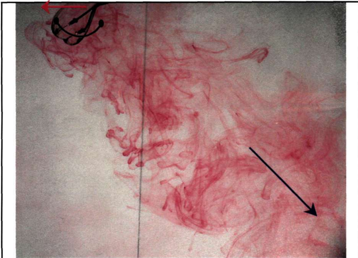
Figure 2.12: In this figure flow field for a flapping wing with asymmetric velocity profiles ( Re=1070-750 ), after many cycles of operations. Unlike in symmetric flapping, in this case asymmetry in the flow field is clearly evident. Almost all the fluid is displaced in the direction of the blue-arrow starting from upper left corner to the lower right corner. As a result, flow from both wings would produce a net lift force in the direction of the red arrow.
