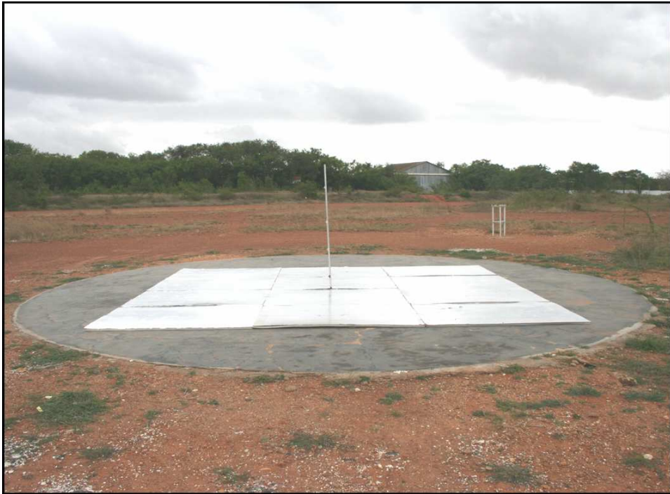
Figure 2.6: A photograph showing the manner in which the concrete patch was covered with panels having aluminium foil as the top surface
