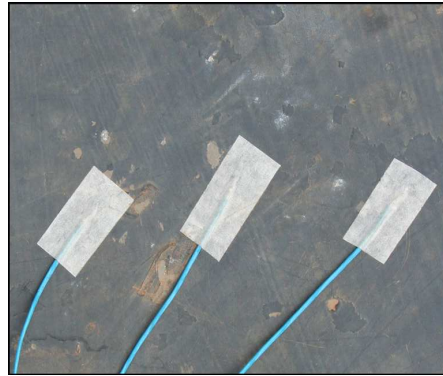
Figure 2.12: A photograph of the manner in which ground temperature was measured using thermocouples. Disc shaped thermocouples (thickness of 0.25 mm) were taped to the ground with a little conducting paste underneath them.
