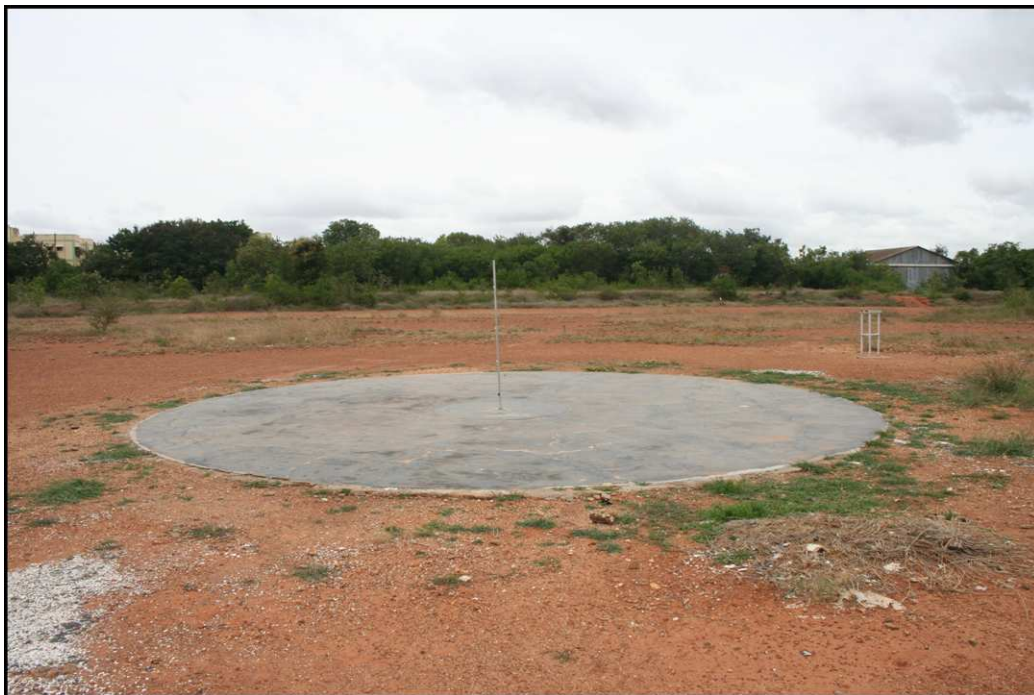
Figure 2.2: A photograph of a closer view of the concrete patch which constitutes the observation site. Also seen is the central mast on which the temperature sensors were mounted.
