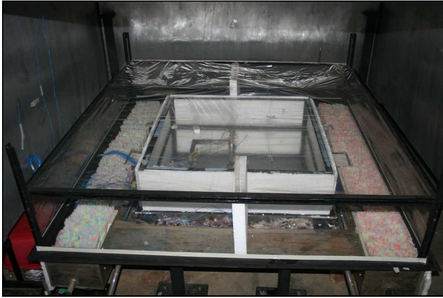
Figure 4.2: A photograph of the laboratory set up. The front ‘outer’ wall has been removed to reveal the test section and air circulation section.
