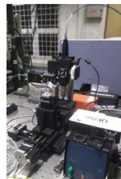
A newly developed portable Raman spectrometer for use in bio-diagnostics under TRC
