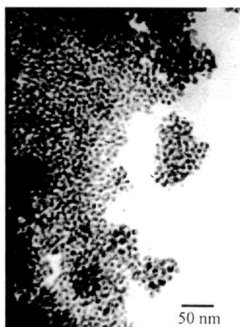
Figure 4.75: Electron micrographs of \sim 7.5 nm Au nanoparticles after interaction with an aqueous 600 \mu\text{M} \text{Cu}^{2+} solution.
