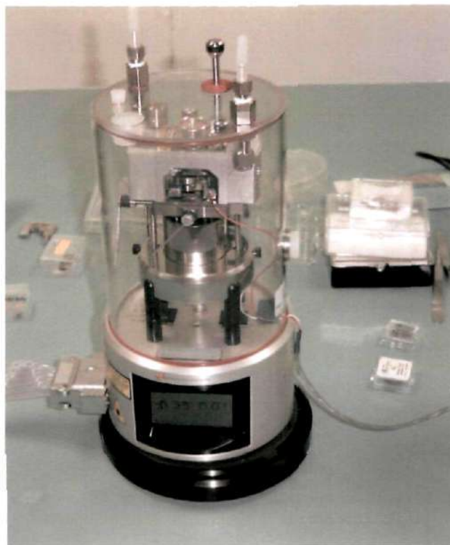
Figure 3.3: Photograph of the atomic force microscope (Digital instruments multimode head).
