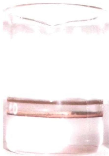
Figure 3.2: Photograph showing a film of Au nanocrystals formed at the interface of water and toluene.
