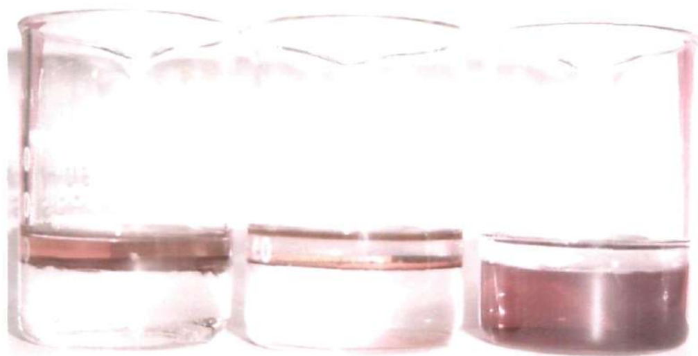
Figure 4.7: Nanocrystalline film of Au formed at the toluene-water interface (middle). Gold is introduced as a toluene solution of \text{Au}(\text{PPh}_3)\text{Cl} while partially hydrolysed THPC (tetrakis(hydroxymethyl)phosphoniumchloride) in water acts as a reducing agent. The film is obtained when the two layers are allowed to stand for several hours. When dodecanethiol is added to the toluene layer, the film breaks up forming an organosol (left) while mercaptoundecanoic acid added to water produces a hydrosol (right).
