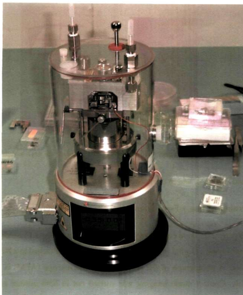
Figure 1.5.4: Photograph of the atomic force microscope (Digital Instruments Multimode head)
