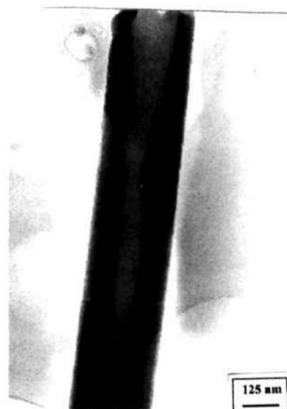
Figure 1.2.34: TEM image of \text{Si}_3\text{N}_4 nanotubes obtained by the reaction of aligned multi-walled nanotubes with silica gel at 1360\text{ }^\circ\text{C} .
