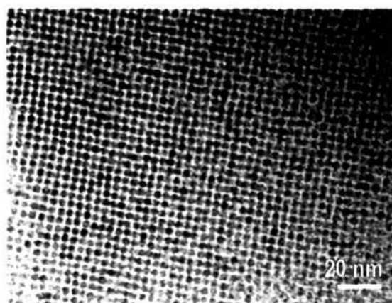
Figure 1.5 Two-dimensional arrays of thiol-derivatised Pd clusters of definite nuclearity. A two-dimensional array of thiol-derivatised Pd-Ni core-shell nanocrystals [11].
