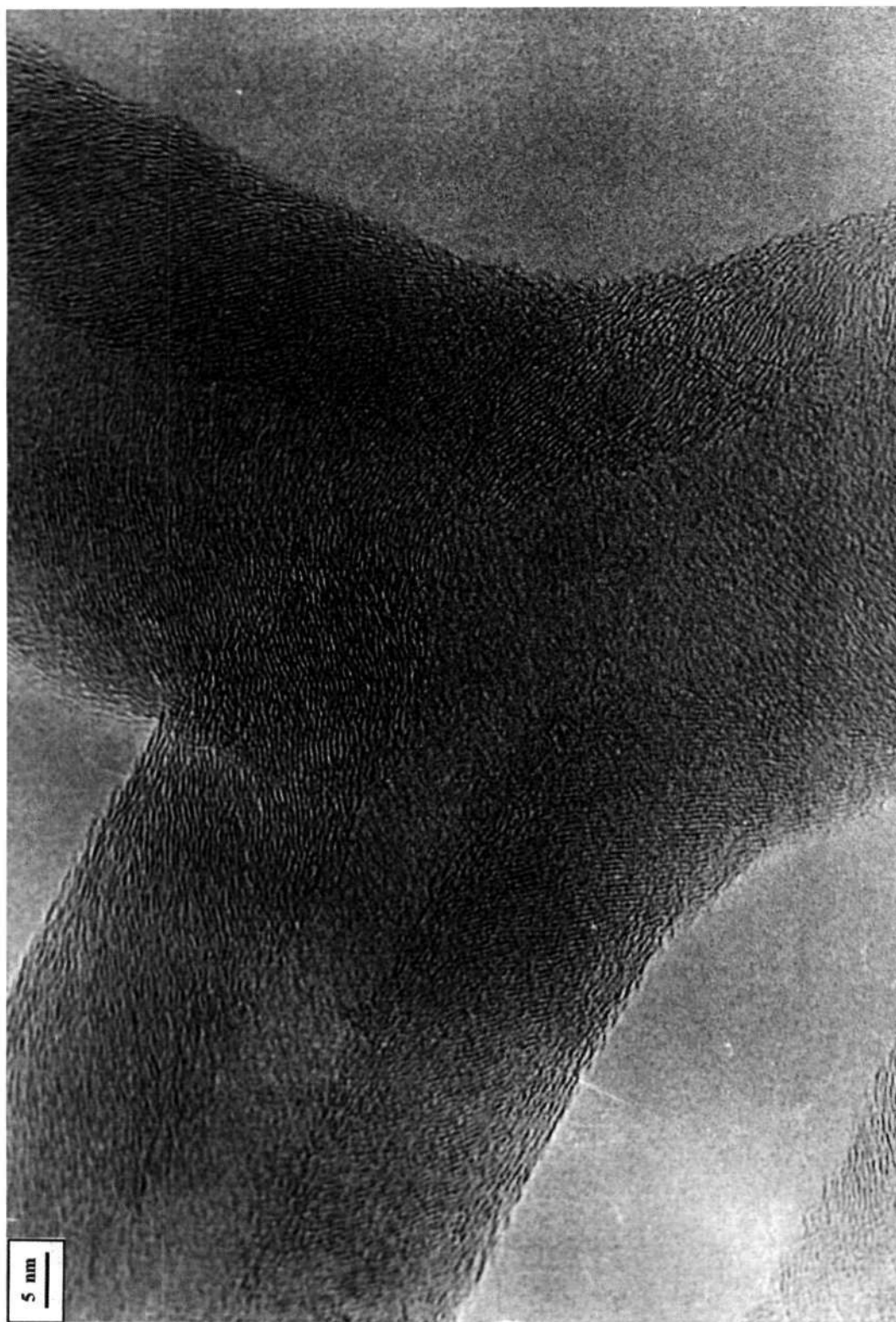
Figure 2.7: High resolution electron microscope image of the Y-junction nanotube obtained by the pyrolysis of cobaltocene-thiophene mixture.
