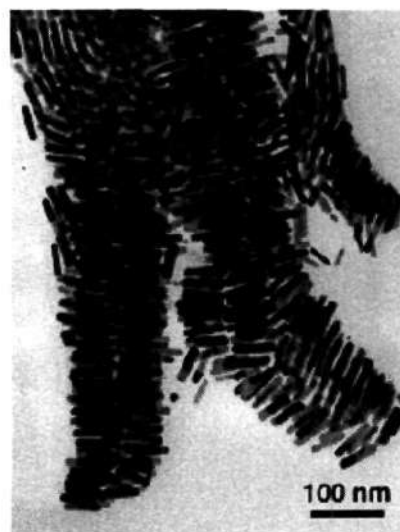
Figure 1.6 Transmission electron micrographs of bundles of DNA-linked gold nanorods. [Ref. 50]
