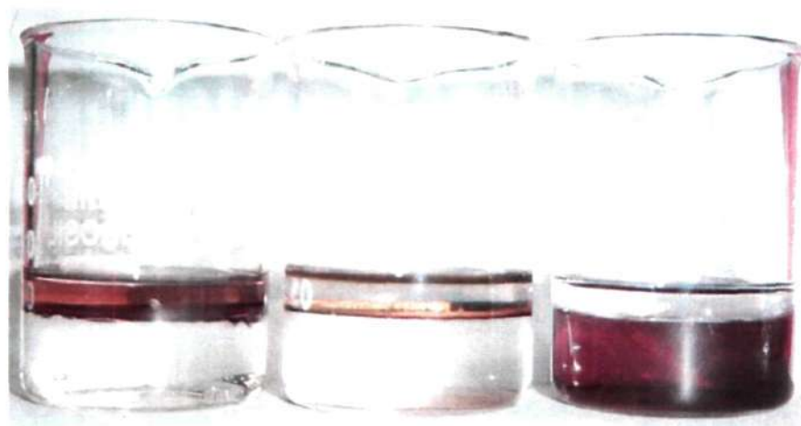
Figure 1.11 Nanocrystalline film of Au formed at the toluene-water interface (middle). When dodecanethiol is added to the toluene layer, the film breaks up forming an organosol(left) while mercaptoundecanoic acid added to water it produces a hydrosol (right) [Ref.80].
