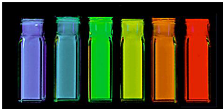
Figure 1.2. Suspensions of CdSe quantum dots under ultraviolet excitation.
