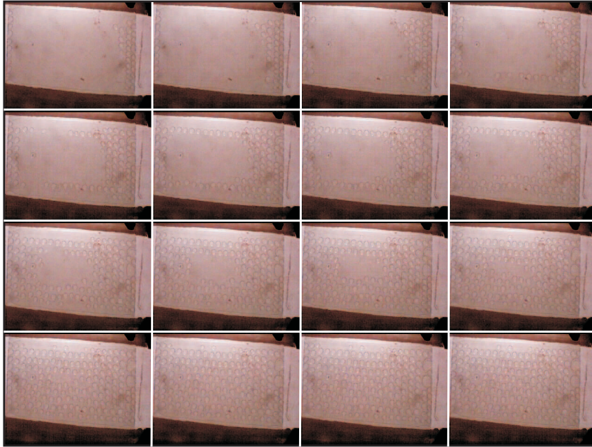
Figure C.1: Frames selected from a video file showing the evolution of pillars. The images represent every 200 th frame. The frame rate of the CCD camera used was 30 fps.
