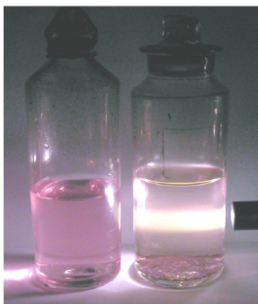
Figure 1.1.2: Gold colloid prepared in 1857 by Michael Faraday (on the right) along with a pink solution (on the left) made by him to resemble the colloids (from [3]).
