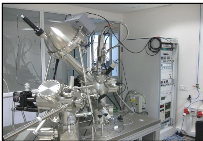
Fig.9 XPS instrument used in the present study – purchased from Bruker, Germany.
