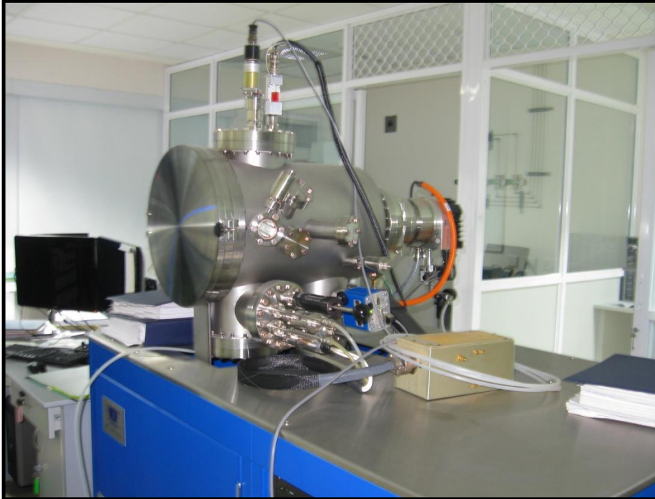
Fig.4 PVD system used in this study- purchased from SVT associates, USA
