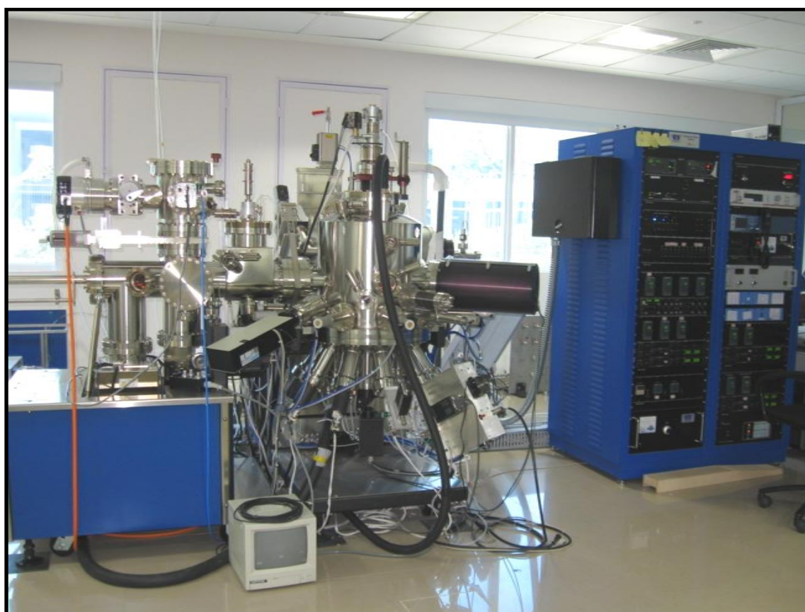
Fig.2 MBE system used in the present study – purchased from SVT associates, USA
