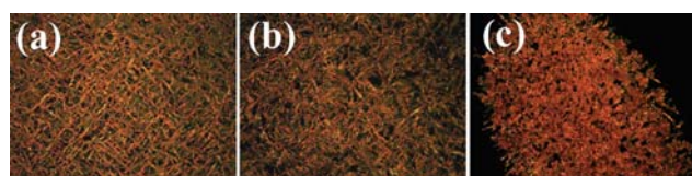
Fig. 6 Different types of birefringent phases for (a) 1 , (b) 1 -Pr-SWNT and (c) 1 - C_{16} -SWNT when cooling from the isotropic phase (1.96 wt% SWNTs added, temperature 125 °C, magnification \times 20 ).
