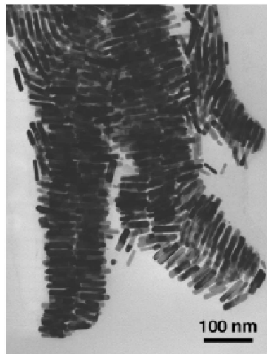
Figure 1.10: Transmission electron micrographs of bundles of DNA linked gold nanorods [109].
