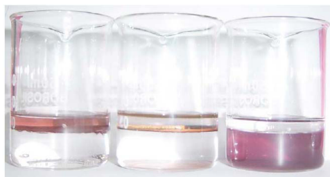
Figure 1.15: Nanocrystalline film of Au formed at the toluene-water interface (middle). When dodecanethiol is added to the toluene layer, the film breaks up forming an organosol(left) while mercaptoundecanoic acid added to water it produces a hydrosol (right) [137].
