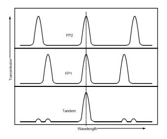
**Figure 2.11.** Elimination of neighboring interference orders in a tandem arrangement of two unequal interferometers.
