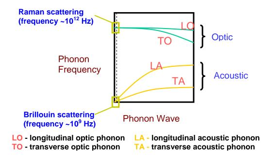
Figure 1.4. Schematic representation of phonon dispersion relation
