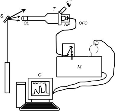
Figure 2.1. Schematic representation of the Raman spectrometer used in the present experiment. S – sample, L – laser, OL – objective lens, T – trinocular, NF – notch filter, OFC – optical fibre cable, D – CCD detector, OC – optical fibre coupling, M – monochromator and C – computer.
