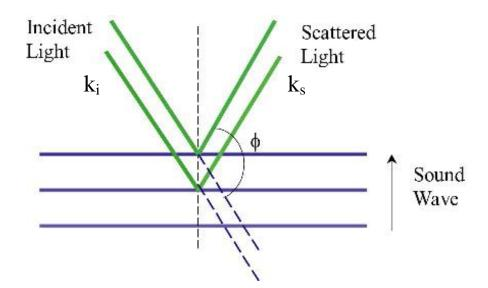
Figure 1.2. Interaction of the sound waves with light.
