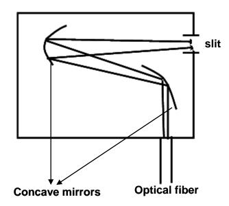
Figure 2.2. f-number matching of the optical fiber with monochromater
