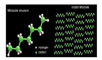
Figure 3.2. Molecular and crystal structure of n-heptane
