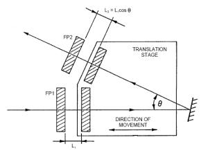
**Figure 2.12.** A translation stage designed to automatically synchronize the scans of two tandem interferometers.
