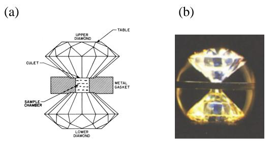
**Figure 2.3.** a) Schematic cross section view of Diamond Anvil, b) Photograph of Diamond anvil
