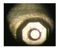
Figure 2.7. Preindented stainless steel gasket used in our experiment
