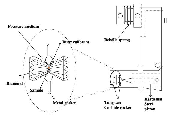
Figure 2.4. Schematic representation of Mao-Bell Diamond Anvil Cell
