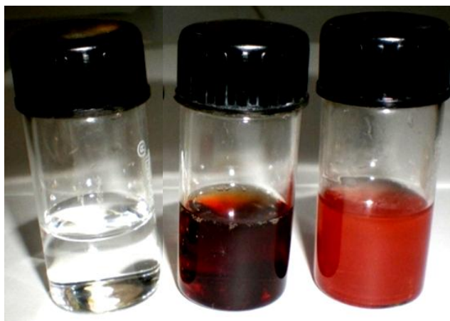
Figure 1. Optical image of aminoclay and Cu-aminoclay solution at different ageing times. From left to right; aminoclay in water, freshly prepared Cu-aminoclay solution (wine-red color) and Cu-aminoclay solution kept for 14 days (brick-red color).
