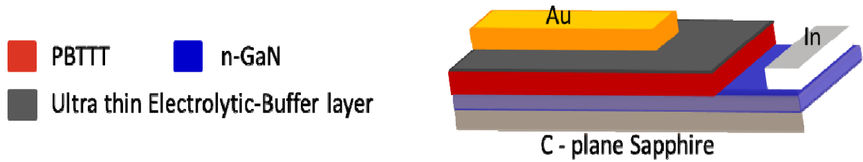
Figure 2.16 : A schematic structure for n-GaN/pBTTT OI hybrid heterostructure device. The pBTTT layer is replaced by other polymers.
