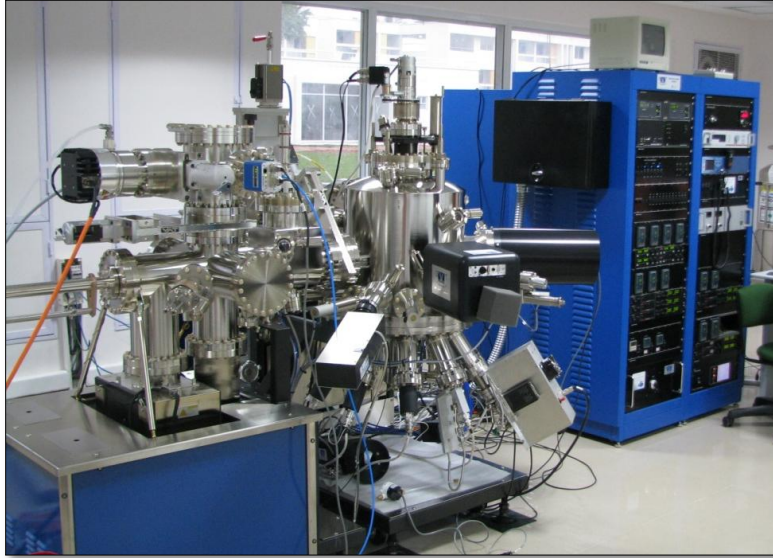
Fig.2.2: SVTA MBE system used in the present study for the growth of GaN nano-structures.
