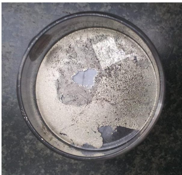
Figure IIIA.19 Photograph of the Ag metal recovered from the crackle coating after liftoff.
