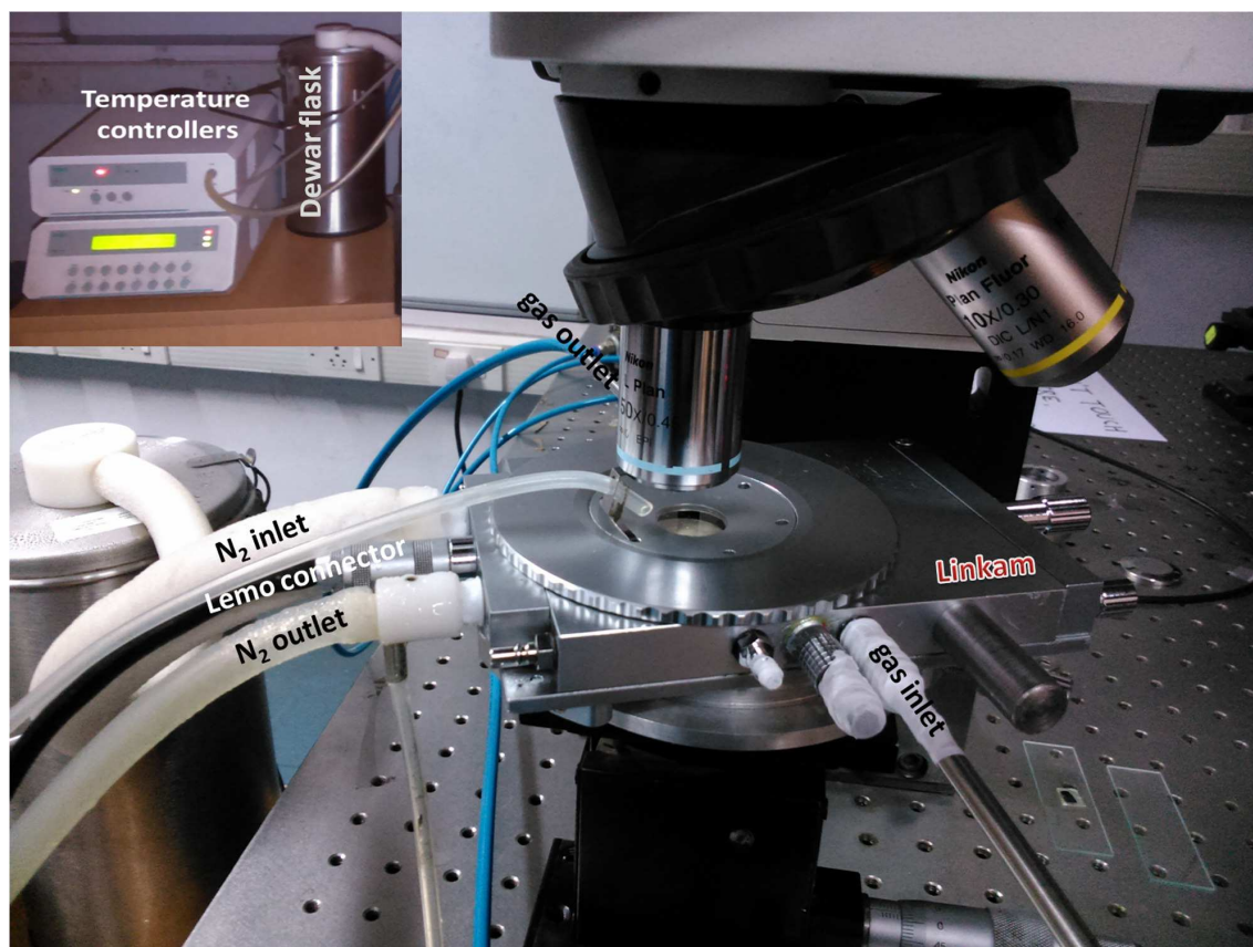
Figure 2.2: Linkam stage employed for temperature dependent and gas adsorption Raman studies of MOFs. Inset shows the temperature controllers and Dewar flask for containing liquid nitrogen.
