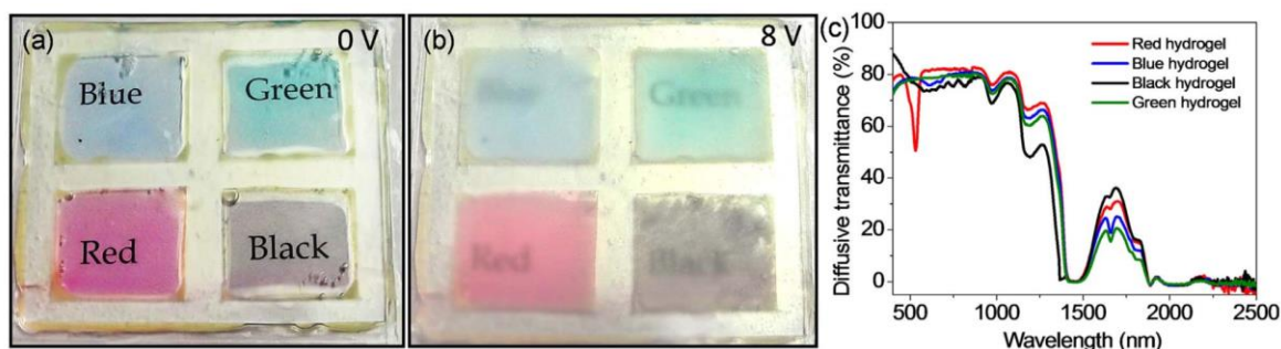
Figure IVA.3.8 Photographs of pixelated color pattern with blue, green, red and black color hydrogels on a TCE in V_{OFF} (a) and V_{ON} (b) states. The diffuse transmittance spectra of different colored hydrogels are shown in (c).
