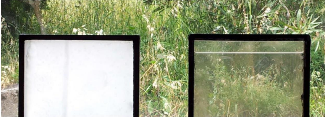
Figure IVB.1.7 PCM glazing windows in opaque solid (left), and transparent fluid state (right).
