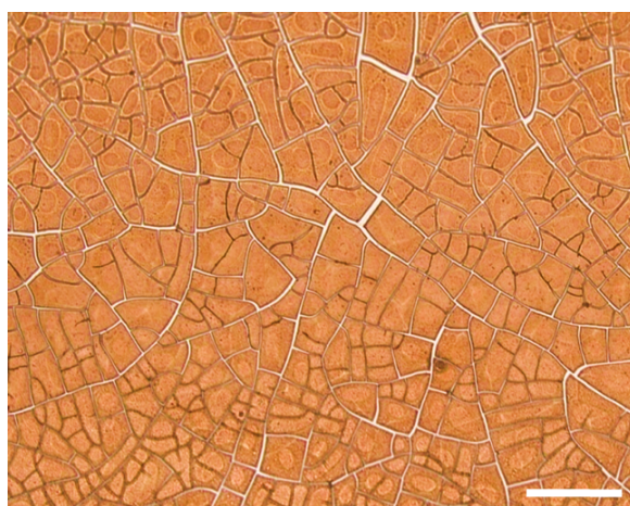
Fig. 3.33 Optical image of cracks formed by using water-IPA mixtures as a solvent instead of only water. Since such mixtures tend to have higher evaporation rates and good wettability, a thickness gradient was not observed in the obtained film. As expected, random cracks rather than parallel cracks were observed to be formed (scale bar 100\ \mu\text{m} )
