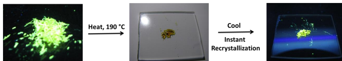
Figure 8. Images of OPE-C gly -A showing melt formation upon heating and instant recrystallization upon cooling.
