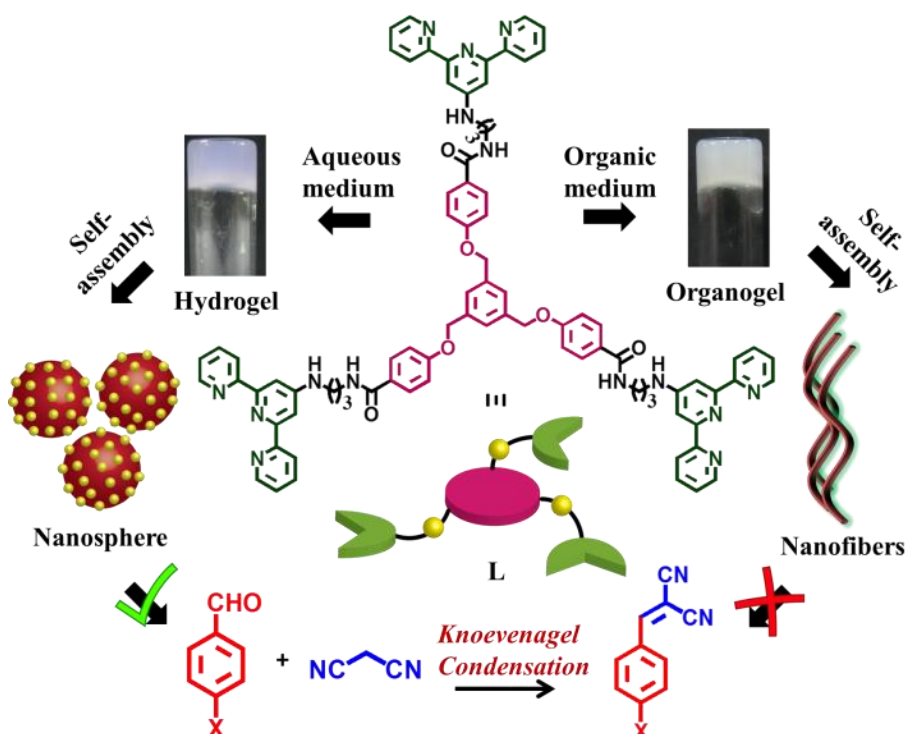
Scheme 1. Schematic showing the self-assembly of L to hydrogel and organogel and their catalytic activity.
