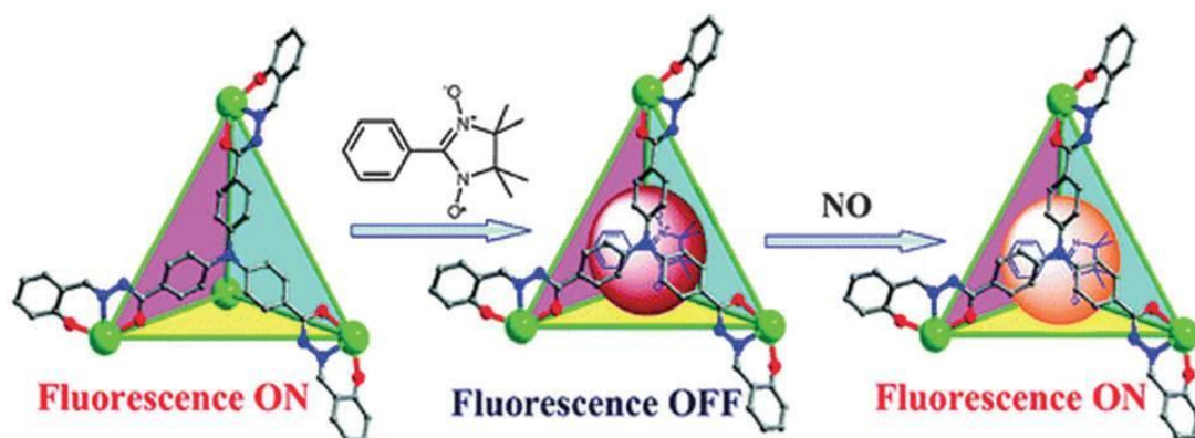
Figure 33. Structure of the Ce-H2TTS functional tetrahedron showing the sequence of fluorescent variation of the tetrahedron upon the addition of PTIO and NO. Figure reproduced from ref. 36a with permission
