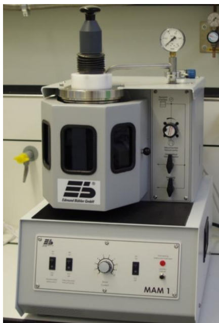
Figure 1.3 MAM-1 Arc Melter designed by Edmund Bühler GmbH.
