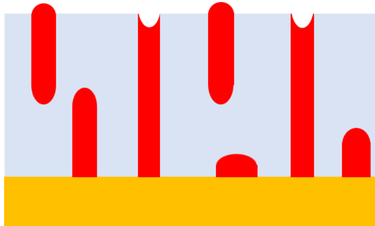
Figure 5.3 Schematic of a ferroelectric memristor adapted from Ref. [15]. In the schematic, red regions indicate SC polymer, and blue regions indicate the FE polymer matrix. Yellow indicates metal electrodes. It can be seen that not all the SC channels bridge bottom and top electrodes.
