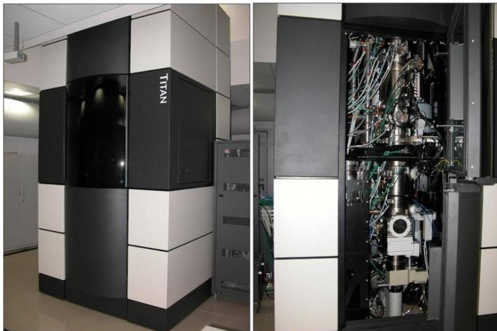
Figure 2.07. FEI TITAN 3 ™ 80-300 kV at International Centre for Materials Science (ICMS), Jawaharlal Nehru Centre for Advanced Scientific Research (JNCASR), Bangalore. It has double Cs corrector technology with both image and probe corrector systems [79].
