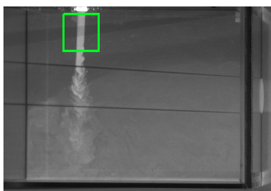
(a) Semi turbulent jet, Re = 1500 , flow rate = 0.489\text{ lpm}
