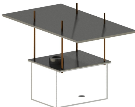
Figure 2.3: Small box with the frame used to suspend it inside the large tank
