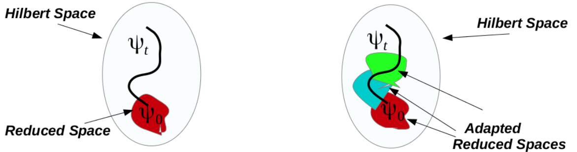
Figure 2.5: Schematic of time evolution of initial state wavefunction, \Psi_0 , obtained from static DMRG method: (a) non-adaptive method i.e. time evolution in the fixed reduced basis. (b) adaptive method, i.e. time evolution in adapted reduced basis.
