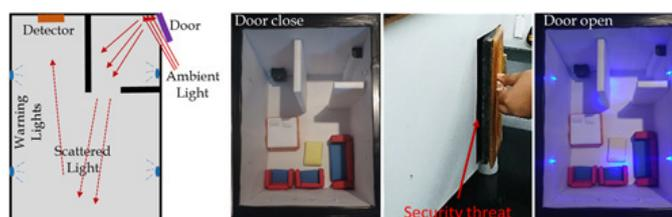
In the prototype, inside the model house, a fabricated detector was mounted beside a high-value commercial detector for comparison and connected to the same external circuit to trigger warning lights (blue lights in the image) and security buzzer. The door is opened to allow only weak scattered light as a sign of unwanted activity. With such low level of lighting, not detectable by the human eye, the fabricated detector was activated, turning on the buzzer and the lights.
