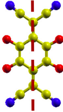
Figure 6.4: Optimized geometry of F_4TCNQ molecule in gas phase. Color code for atoms: red (F), yellow (C), and blue (N). The long axis of F_4TCNQ , which passes through C atoms attached to CN^- groups, is shown using a dark red dashed line.
