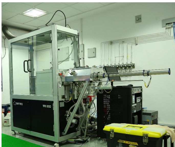
Figure 2.5 A photograph of Beneq TFS-200 ALD system installed at JNCASR, Bengaluru, India
