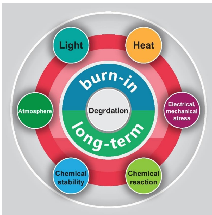
Figure.1.23. Infographic depicting the various factors causing degradation in organic solar cells.
