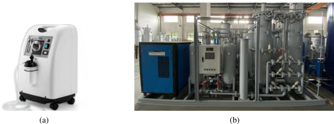
Fig. 1.4 Adsorption based oxygen separation device (a) Portable oxygen concentrator (b) 100-1000 sLPM PSA plant
