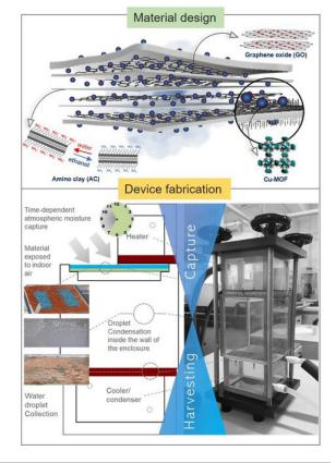
The schematic of material preparation and prototype developed by JNCASR team
