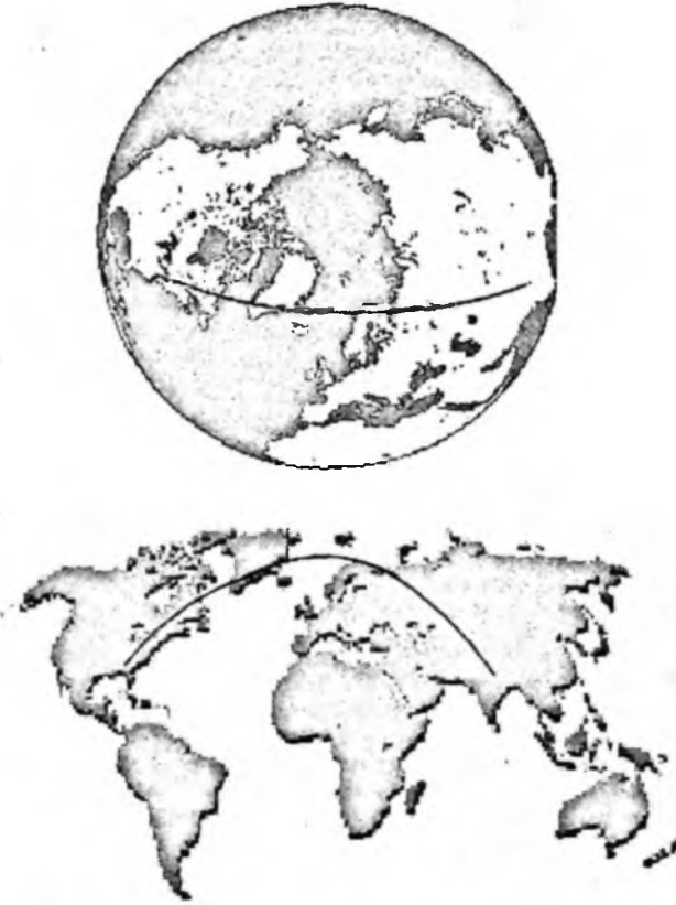
Fig. 2.4 The shortest path on the curved face of the Earth will appear to be curved when described on a map drawn on plain paper, as shown by the appearance of the same path – the shortest path between New Delhi and Washington D.C. – on the surface of the round Earth (top) and on plain paper (bottom).
