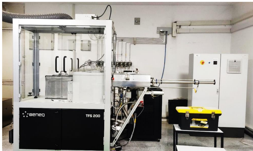
Figure 8: Photograph of Beneq TFS-200 ALD system.
